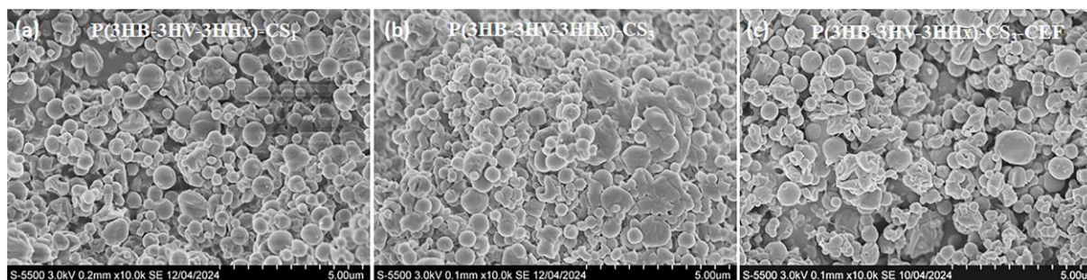
Figure 2. SEM images of chitosan-modified P(3HB-3HV-3HHx) microparticles: (a) P(3HB-3HV-3HHx)-CS 1 ; (b) P(3HB-3HV-3HHx)-CS 3 ; (c) P(3HB-3HV-3HHx)-CS 3 -CEF. The decoding of analyzed microparticles is presented in Table 2. The bar is 5 \mu\text{m} .
