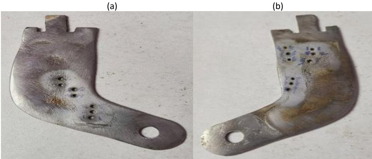
Figure 2. Machined EOS stainless steel 316L with (a) 7 holes and (b) 9 holes
