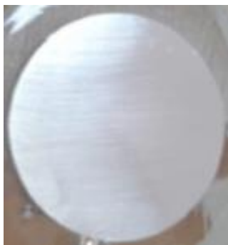
Figure 9. Surface image of three layers of waterborne acrylic coating C1 coated on a RG7 bronze where each layer was dried at 40 °C for 4 hours
