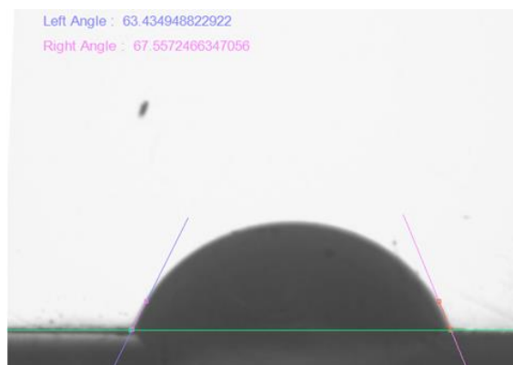
Figure 4. Wetability test of IL-MoO 3
