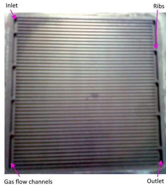
Figure 3. Engraved serpentine gas flow channels in bipolar plate
