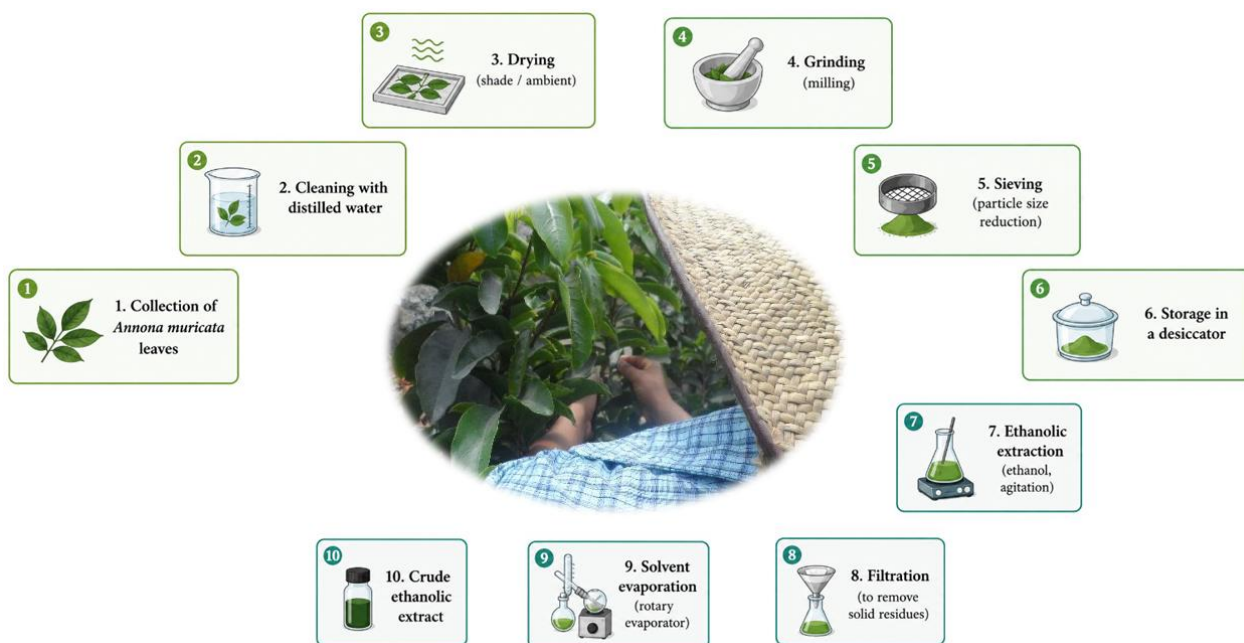
Figure 1. Schematic representation of the preparation of Annona muricata leaves and the subsequent ethanolic extraction procedure used to obtain the crude plant extract employed as a green corrosion inhibitor
