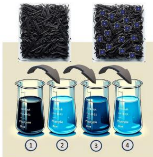
Figure 2. The self-assembly of the (MWCNT/NiTsPc) n film in 4 states and the photograph for the desired structuration of the MWCNT and NiTsPc molecules distributed on the ITO substrate [73], originally published under a BY NC ND 4.0 license
