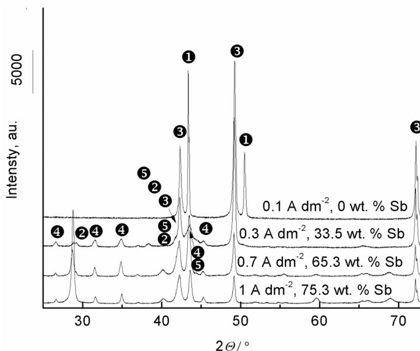
**Figure 5.** X-ray diffractograms of Cu-Sb coatings with different antimony content, obtained in the electrolyte, presented in Table 1. The existed phases are marked with numbers 1 - Cu; 2 - Sb; 3 -  $\text{Cu}_{2.6}\text{Zn}_{1.4}$ ; 4 -  $\text{Cu}_2\text{Sb}_1$ ; 5 -  $\text{Cu}_{11}\text{Sb}_3$
