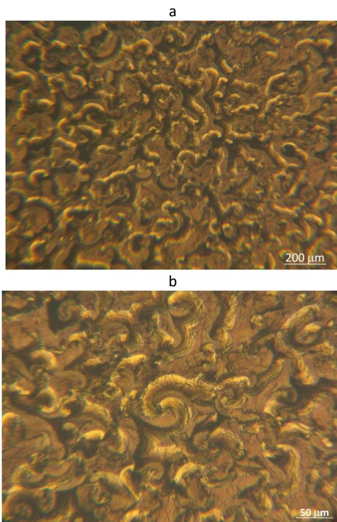
**Figure 6.** Optical images of the coating at different magnifications with spatio-temporal structures, obtained at:  $j = 0.4 \text{ A dm}^{-2}$ , deposition time- 240 min, thickness  $\sim 23.76 \mu\text{m}$
