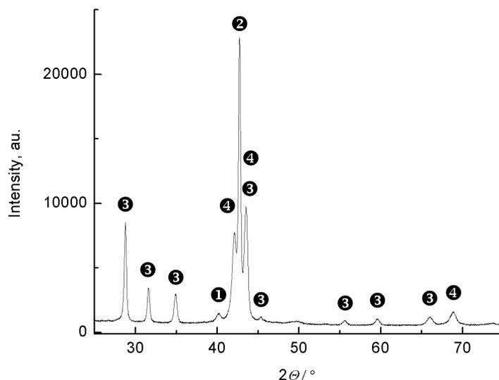
**Figure 7.** X-Ray diffractogram of the sample, shown in Figure 6. The registered phases are marked with numbers: 1 – Sb; 2 – Cu<sub>2,6</sub>Zn<sub>1,4</sub>; 3 – Cu<sub>2</sub>Sb<sub>1</sub>; 4 – Cu<sub>11</sub>Sb<sub>3</sub>.
