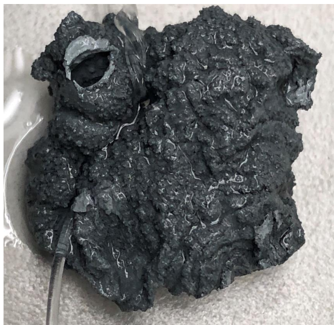
Figure S-25. Aluminum 5052 after 100 min of immersion in 4 \text{ mol L}^{-1} \text{ KOH} + 0.2 \text{ mol L}^{-1} \text{ ZnO}
