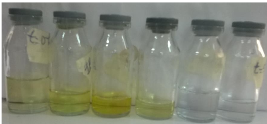
Figure 14. photo of the solution withdrawn from the wastewater tank during electrolysis (from left to right : t = 0 h; 1h; 2h; 3h; 4h; 5h)
