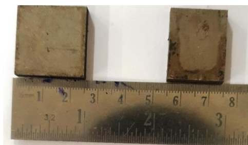
Figure 1. SS-304 substrates obtained after WEDM cutting
