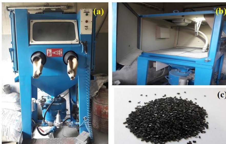
Figure 2. (a) Front and (b) side view of shot blasting machine and (c) blasting medium
