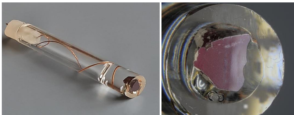
Figure 3. Overall structure of a CG electrode, diameter 12 mm, length 9 cm (left), glass surface (right)
