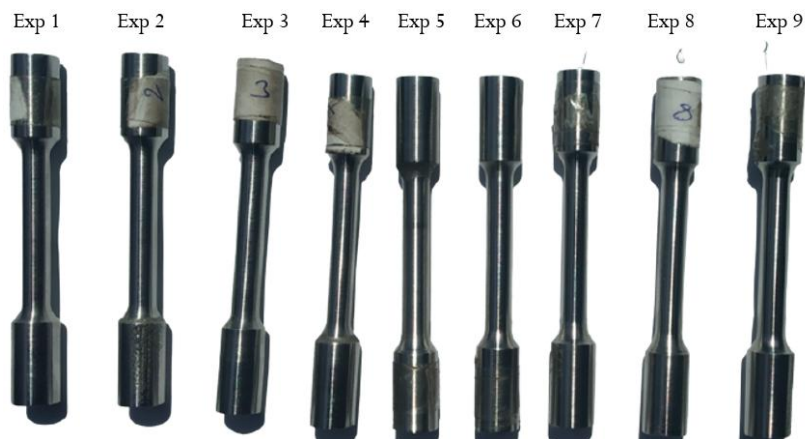
Figure 3. Tensile test specimens in L9 experimentation
