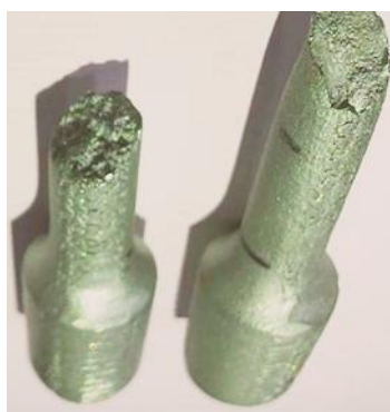
Figure 8. Specimens after tensile test
