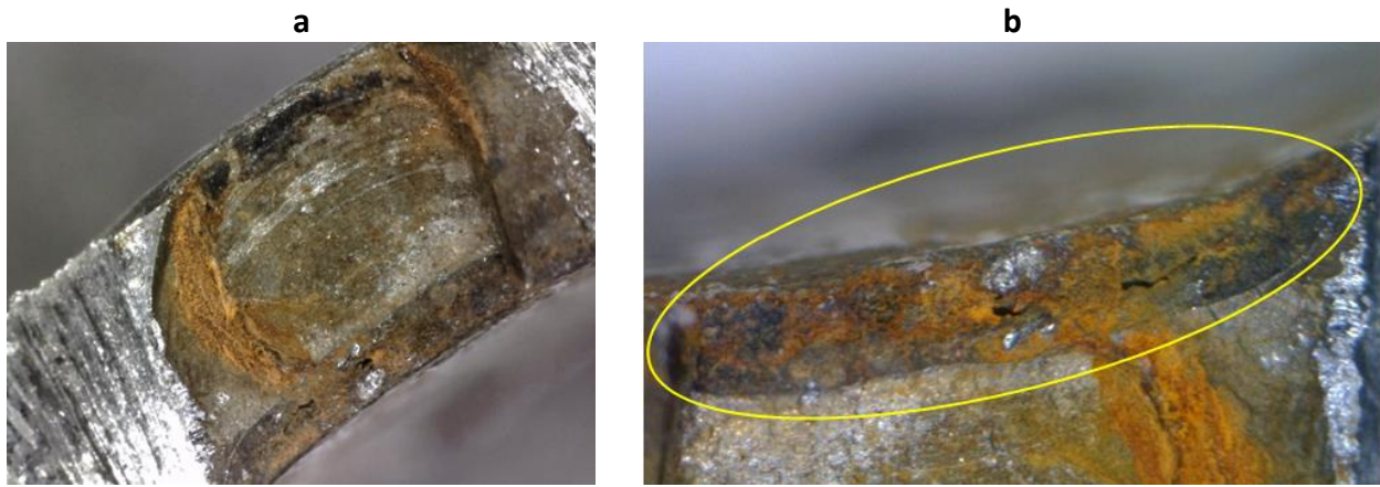
Figure 5. Light microscope photographs of a - fracture surface and b - fracture initiation site
