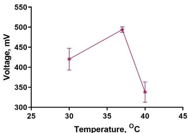
Figure 8. Effect of temperature on voltage generation.
