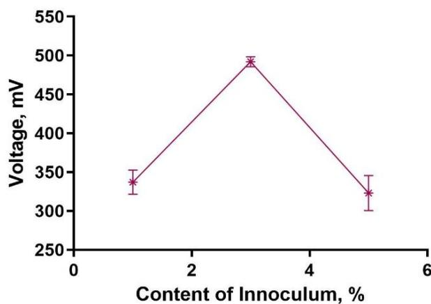
**Figure 7.** Effect of inoculum content on voltage generation.
