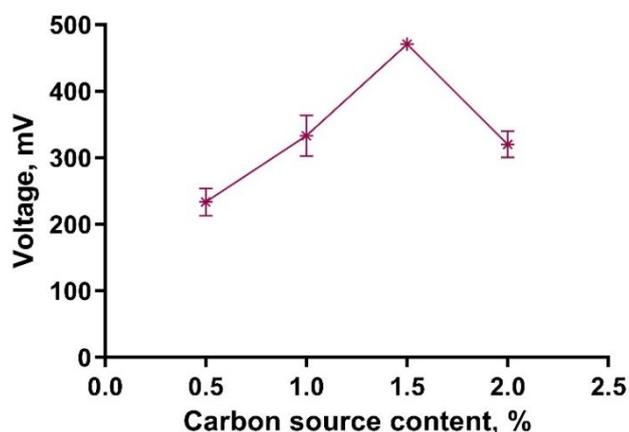
**Figure 4.** Effect of carbon content (lactose) on voltage generation
