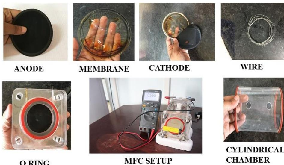
**Figure 1.** Single-chamber MFC components and setup
