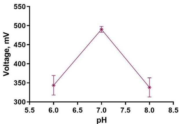
Figure 9. Effect of pH on voltage generation
