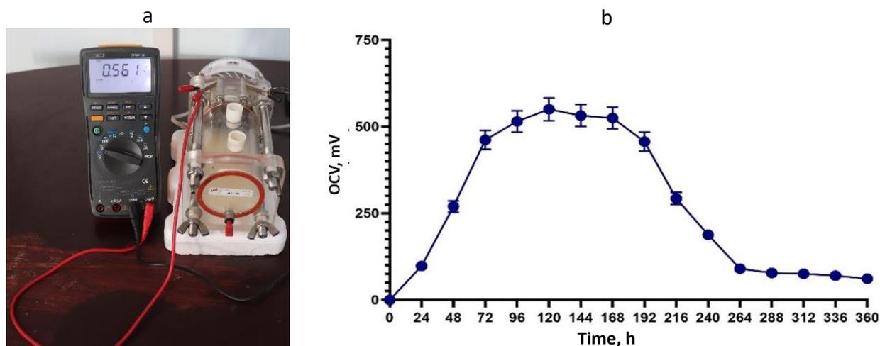
**Figure 11.** (a) Maximum voltage reached in batch operation of MFC with real dairy wastewater; (b) voltage vs. time in batch operation of MFC with real dairy wastewater
