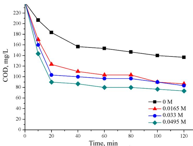
Figure 5. COD removal vs. treatment time at 0.5 A of wastewater samples containing 0.01M NaCl, pH 3, and different concentrations of H<sub>2</sub>O<sub>2</sub>
