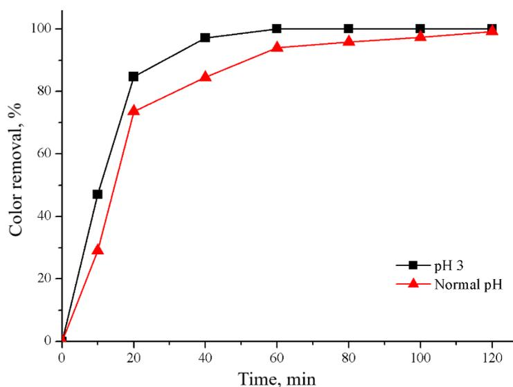
**Figure 2.** Decolorization efficiency vs. treatment time at 0.5 A of wastewater samples containing 0.033 M  $\text{H}_2\text{O}_2$  and 0.01 M NaCl, at pH 3 and 6.8
