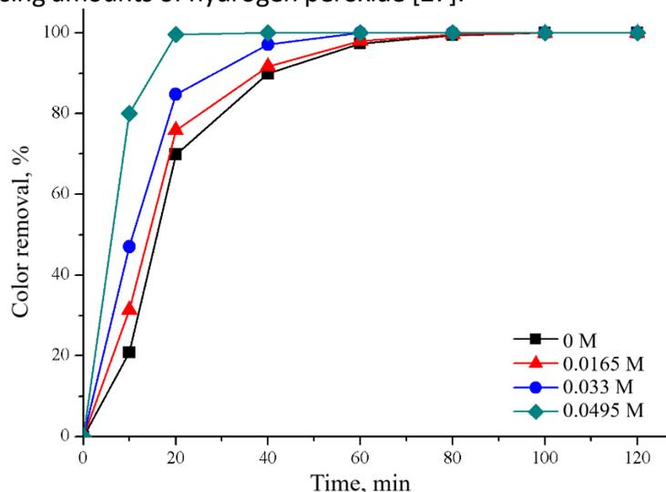
Figure 4. Decolorization efficiency vs. treatment time at 0.5 A of wastewater samples containing 0.01 M NaCl, pH=3 and different concentrations of H<sub>2</sub>O<sub>2</sub>
