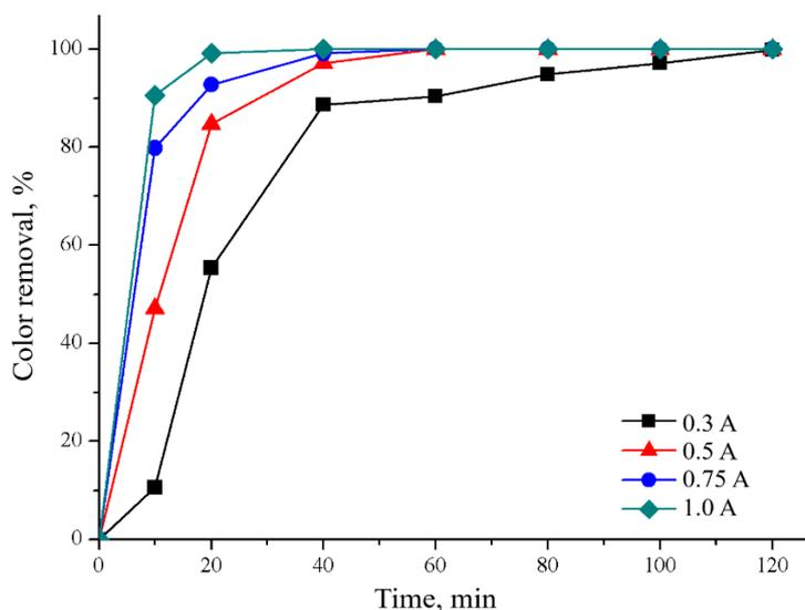
**Figure 6.** Decolorization efficiency vs. treatment time of wastewater samples containing 0.033 M  $\text{H}_2\text{O}_2$  and 0.05M NaCl, pH 3 at different current intensities
